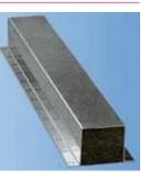
The figure here below shows the result on omega shape with spot welded joints for HLSA, mild steel and stainless steel 301 type (301L) 2B and temper rolled conditions.
